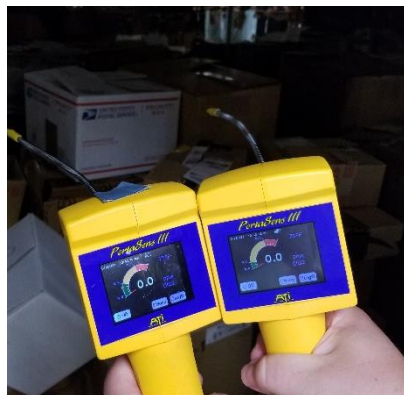
Figure 3: Measurement of CD off gassing inside chamber after opening the door (left) and also inside 1 box (right). 0.0PPM was measured on both locations.
