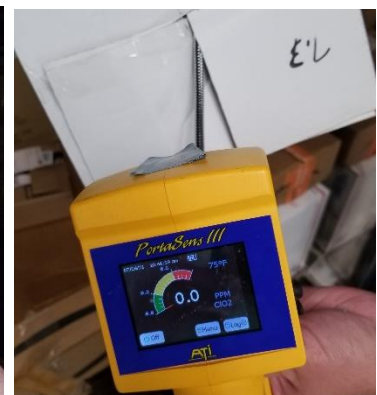
Figure 3: Measurement of CD off gassing inside chamber after opening the door (left) and also inside 1 box (right). 0.0PPM was measured on both locations.
