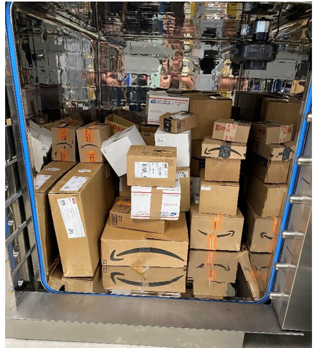
Figure 1: Pallet sterilizer filled with 27.2lbs (12.34kg) of various corrugated cardboard boxes.
