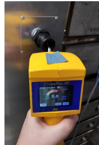
Figure 2: Measurement of CD off gassing 30 minutes post aeration with chamber door closed and NO exhaust on. 0.0 PPM was measured using both sensors.
